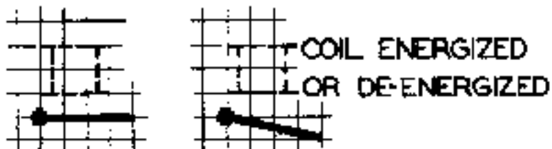
NEUTRAL FRONT CONTACT CLOSED OR OPEN
