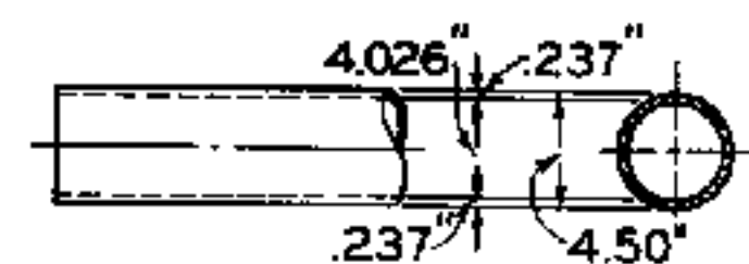
4 INCH PIPE SECTION WROUGHT IRON OR STEEL
