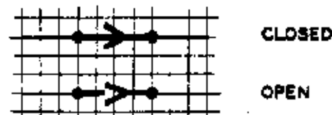
BRIDGE CIRCUIT CONTROLLER
