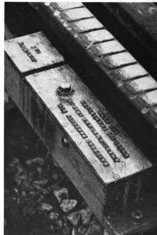
Car wheels traveling over notches in rail set up vibrations for speed sensing.
