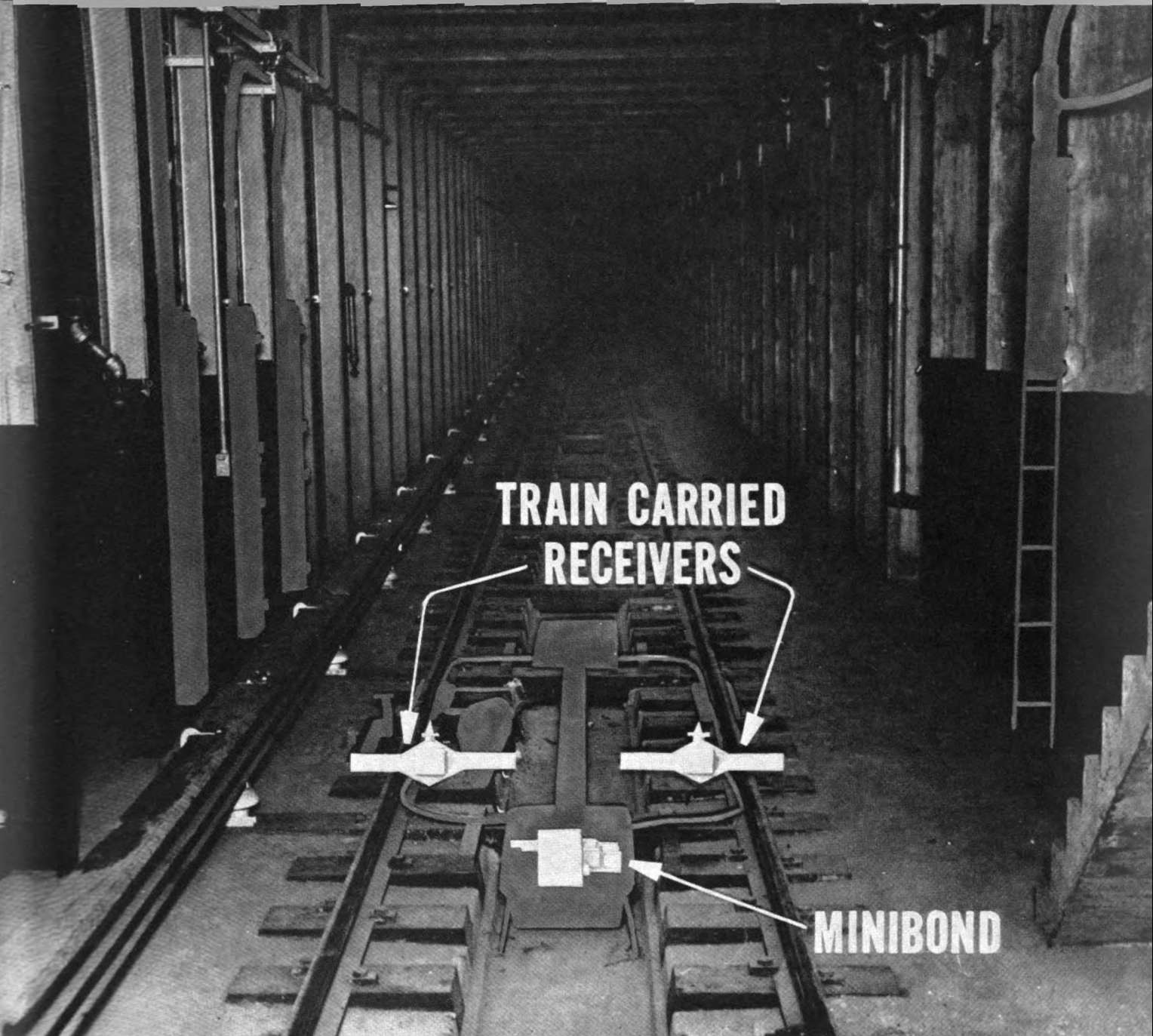
New miniature impedance bond could be mounted between the rails in an existing subway.
