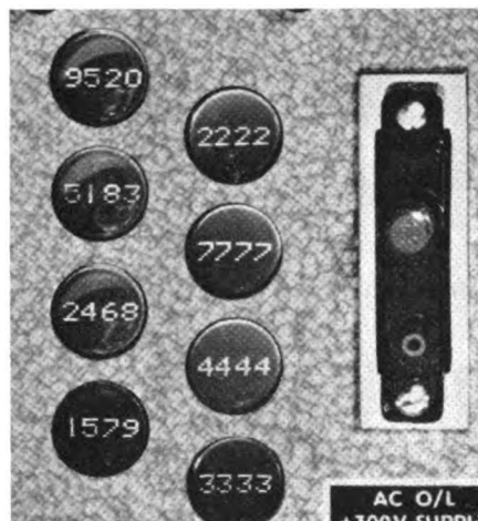
Cathode ray tube type indicators show how characters are formed.
