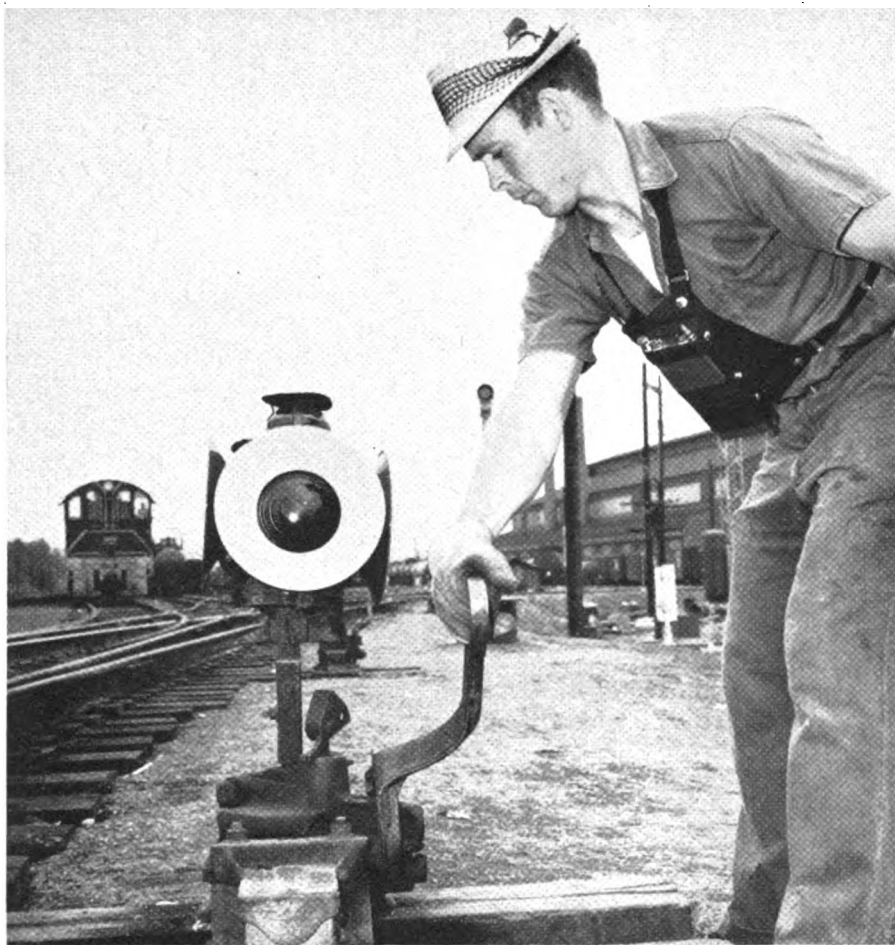
Two-way radio in chest harness lets crewman have hands free to work.
