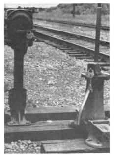
be provided and locking may be released either automatically, or by thcontrol operator, but only after the control circuits of signals governing movement in either direction over the switch and which display aspects with indications more favorable than "proceed at restricted speed" have been opened directly or by shunting of track circuit.
