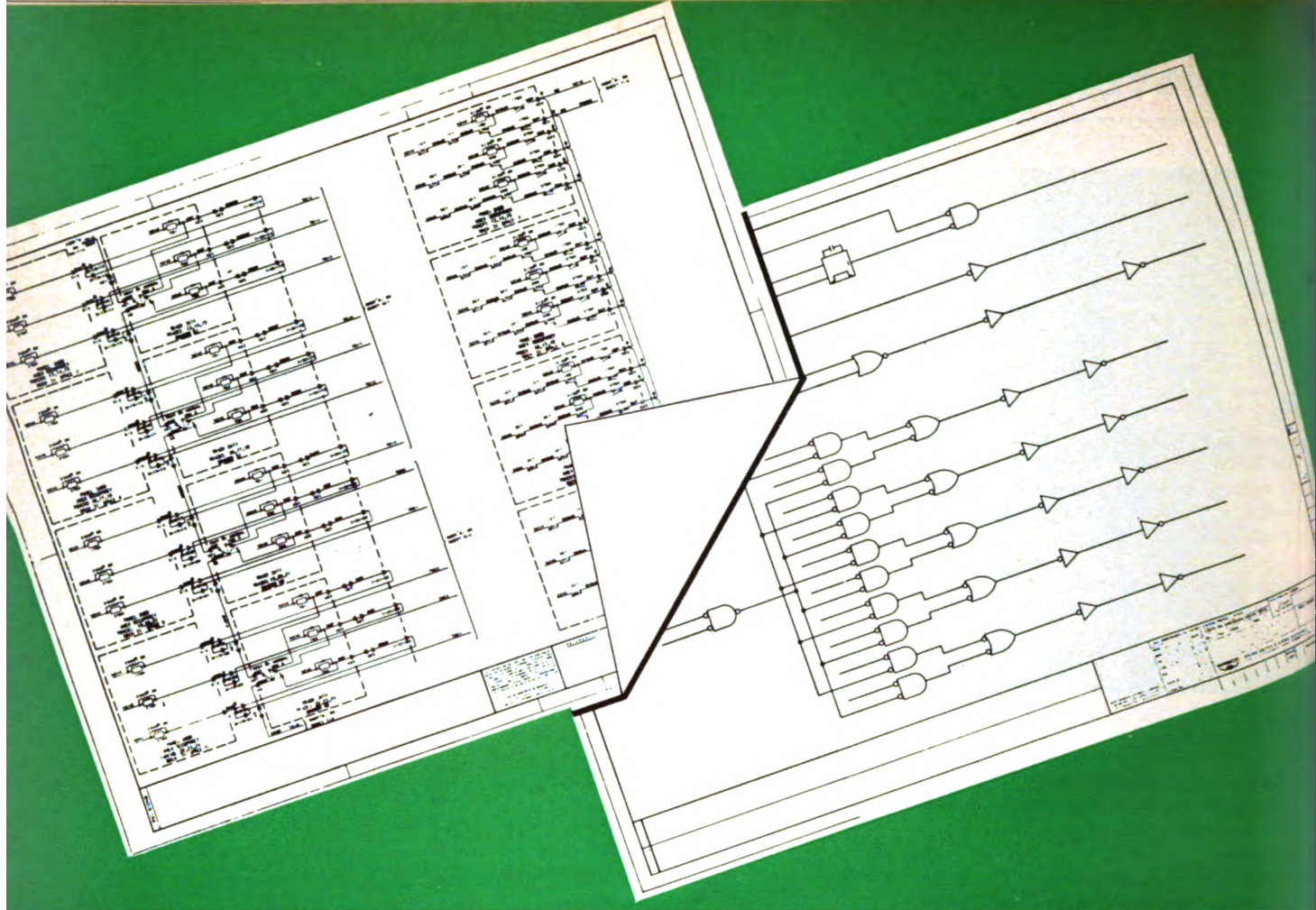
Computer vs Relay: Logic diagram for a computer (right) is equivalent to the circuit diagram for a relay system (left).
