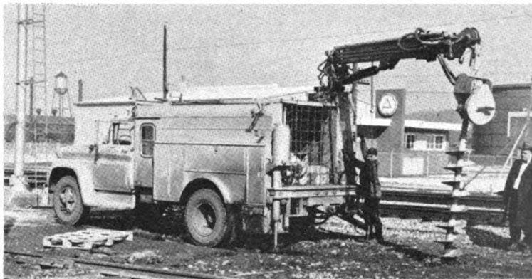
Cherry picker can be used to dig line pole holes, foundation holes or carry an insulated bucket for high-level work.
