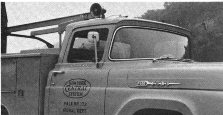
Signal maintainers' trucks have outside loudspeaker that broadcasts radio calls when maintainer is out of truck.
