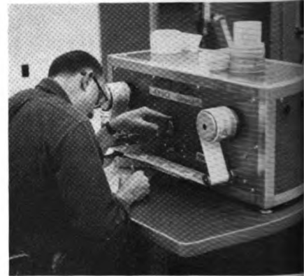
Car checker in yard office moves train picture tape by foot controls, leaving hands free to check consist list.
