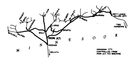
CTC territory (above) connects many important iron ore mines and train assembly yards. TCC machine (below) has pushbuttons for selecting controlled locations, and operating switches and clearing signals.
