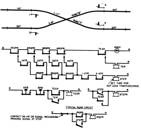
relays than others. In some cases as many as five thermal relays are used, each with a repeater, to provide loss of shunt protection as required under ICC rule 136.309. After extensive study and experimenting with various circuits, I came up with the scheme shown. Since there are still automatic interlockings to be installed, and some so obsolete that it might be economical to rewire them completely, I thought others in the signaling field would be interested in them.
