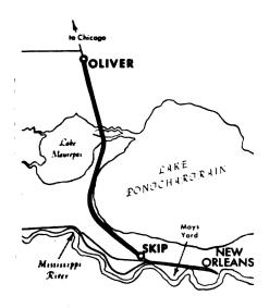
**Above:** Centralized traffic control in this project extends 37 miles from Skip to Oliver with the control machine at Mays Yard, New Orleans. This section includes the longest continuous curve in the U.S., 9.45 miles.
