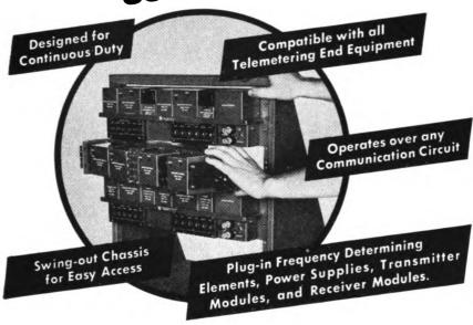
The Model 1220 and 1220A Carrier Terminals are completely transistorized and may be operated from station batteries from 12 to 130 DC. Plug-in power supply is available for 115-volt AC operation. All components, including amplifiers, frequency determining components, and power supplies are contained in plug-in modules, and may be readily interchanged. As many as 22 high-speed channels are available between 300 to 3000 cps.
