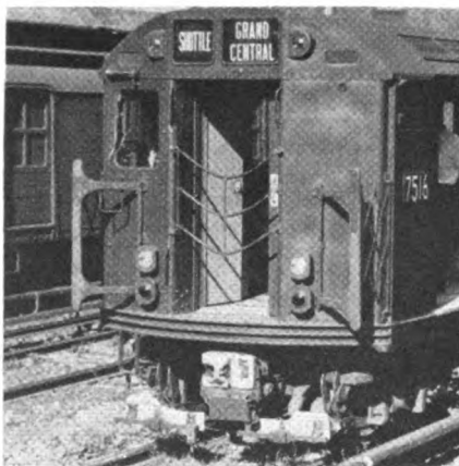
Application of 75 code to a wire loop with train at station controlled doors to open. Train is at 18th Ave. station. Receivers and control equipment (right) are USGS at this end of the train.
