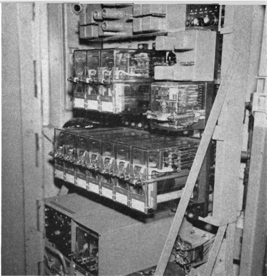
Control equipment is mounted in the rear motorman's compartment of each leading car. Motorman's control in the forward cabs will be for operation when not on the shuttle.
