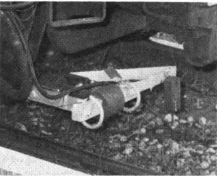
Receivers (above) and controls (top photo) are GRS. Receiver coils are encapsulated in an epoxy resin.
