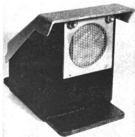
A cast iron case houses the radiometer head at trackside.
