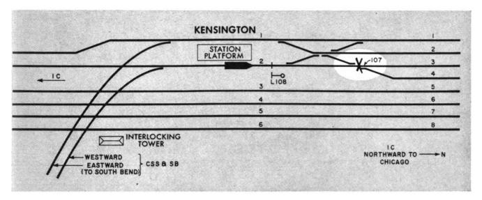
ing protection afforded switch No. 107 when he moved the interlocking machine lever controlling that switch, thereby causing the derailment.
