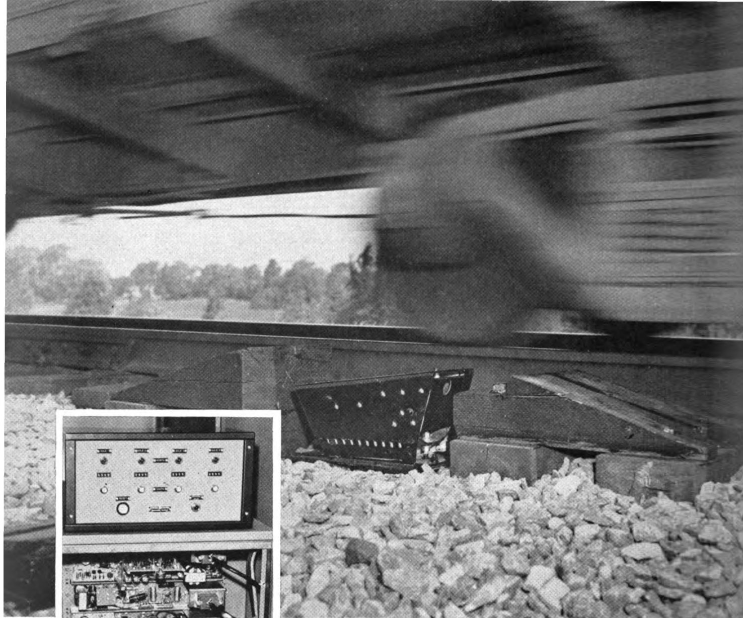
Hotbox detector views journal for one ten-thousandth of a second. Indications are sent 65 miles to dispatcher's office where hotbox indication alarm equipment (inset) registers up to four hot journals on a train.
