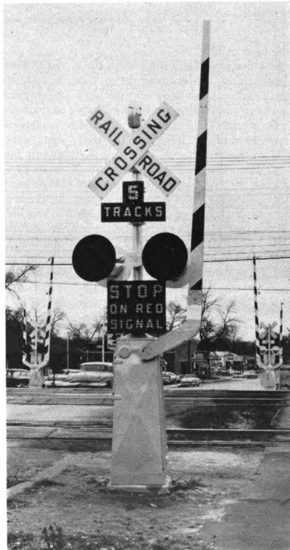
At one-way streets, sidewalk gate is used. When making repairs, swivel base of gate mechanism enables maintainer to swing lowered arms out of the way.
