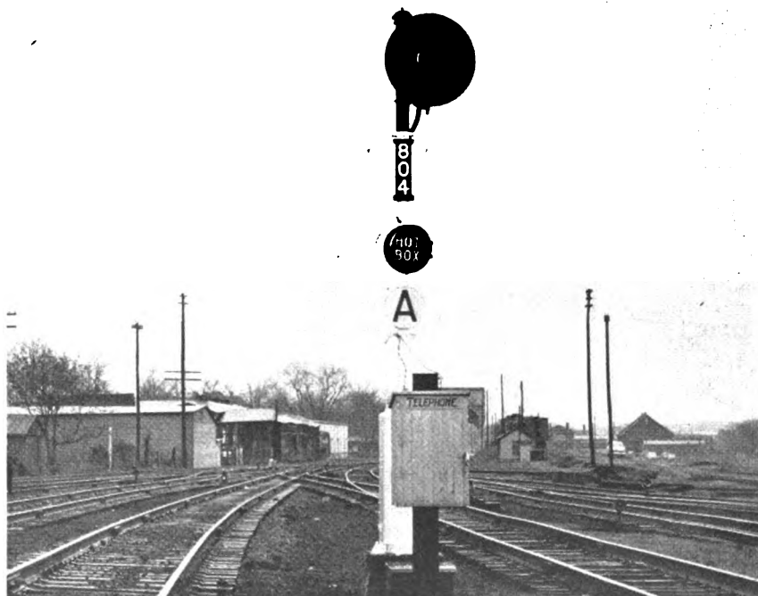
3 . . . pip for a hot box, sets signal to Red; hot box marker is lighted.
