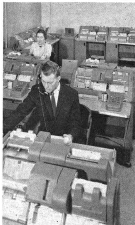
Car-Fax headquarters at Chicago is where all reports from the 68 field stations or mechanized yards come in via transceiver network. Up to four field stations can be handled simultaneously on one transceiver circuit. The transceivers operate at the rate of 10 cards per minute. It takes only 10 to 15 minutes to handle a train consist.
