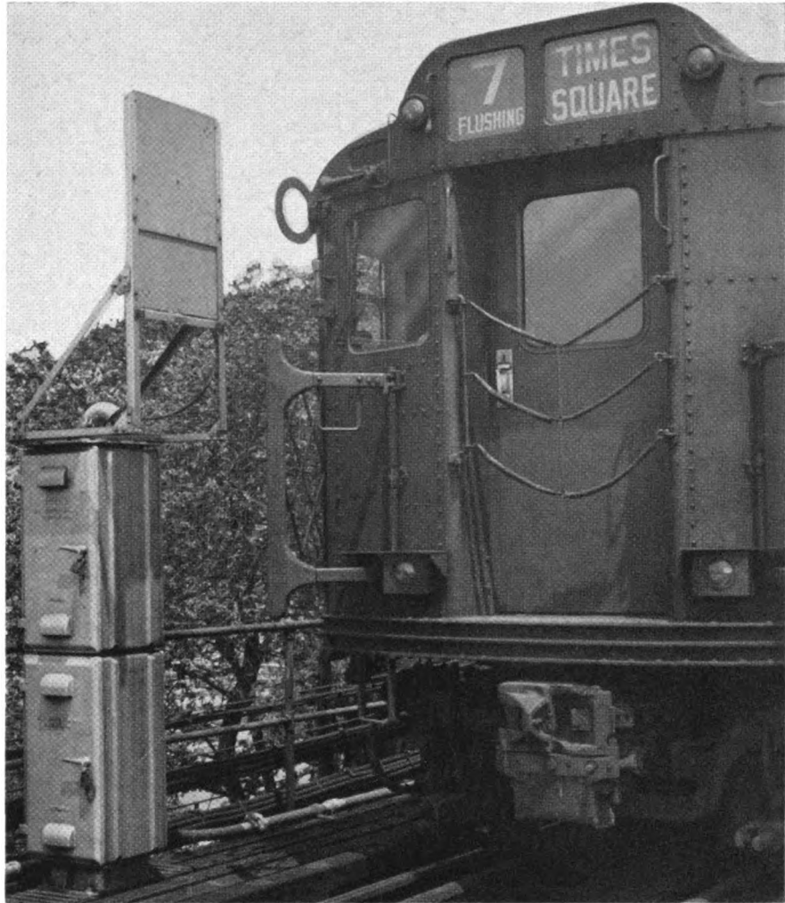
City-bound train initiates calls for trailing-point switches at Rawson street
