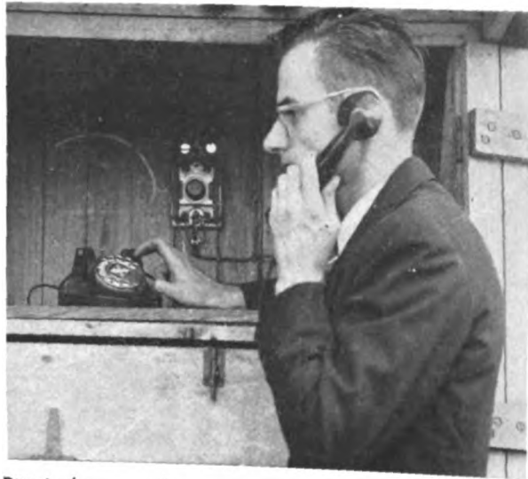
Due to low annual cost of railroad-owned automatic phones they can be installed at many places
