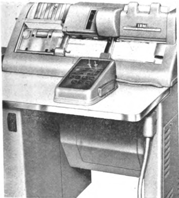
Data transceiver "reads" a punch card, transmitting data over voice circuit to like unit that punches a new card
