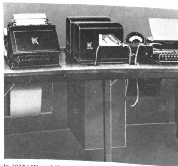
In 1914 L&N used Kleinschmidt teletypewriters and 1920 saw keyboard punch, automatic transmitter and page printers
