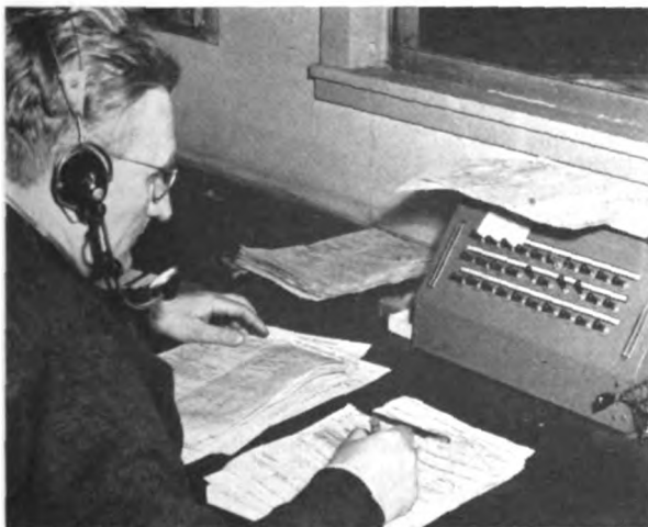
This checker's console has lines to all outlets in house
