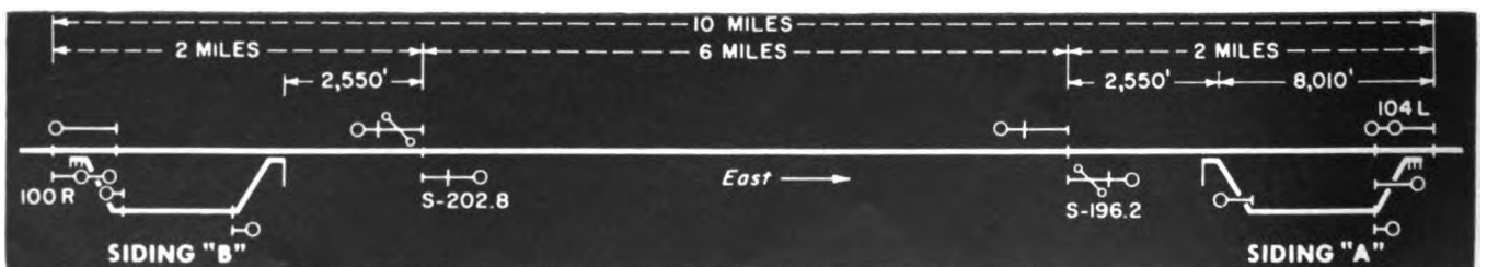
Fig. 2 CB&Q uses spring switch at end and power switch at other end of siding
