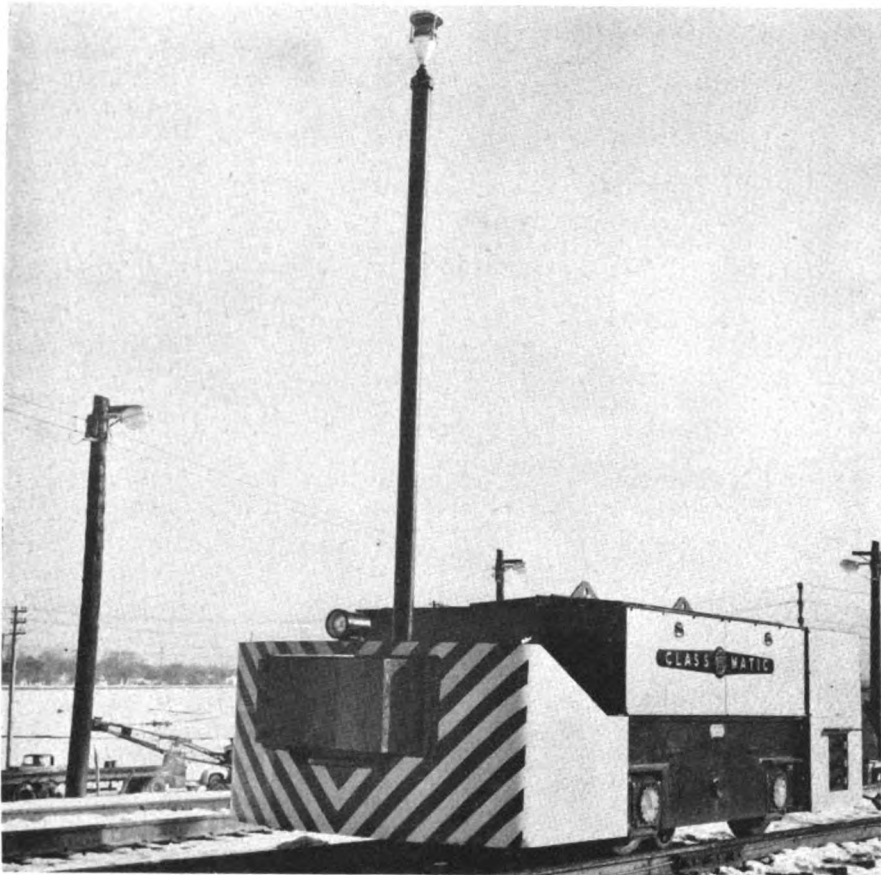
Yard accelerator is unattended unit to push cars to clearance on class tracks
