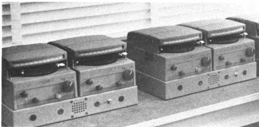
Recorders are paired for car checking so no cars are "missed" in a long train
