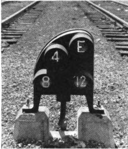
Stop-pushing signal indicates car lengths to go to clearance point
