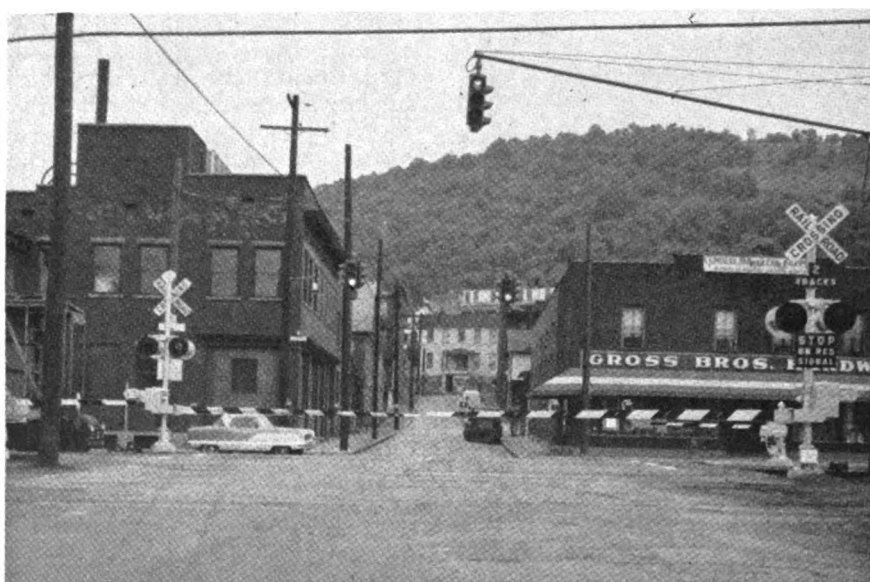
Knox street looking north. Traffic light in foreground is red, while two lights in back over Henderson avenue are green to permit cars to move off crossing
