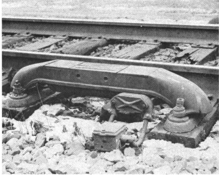
. . . . rides over wayside inductor used also for automatic train stop
