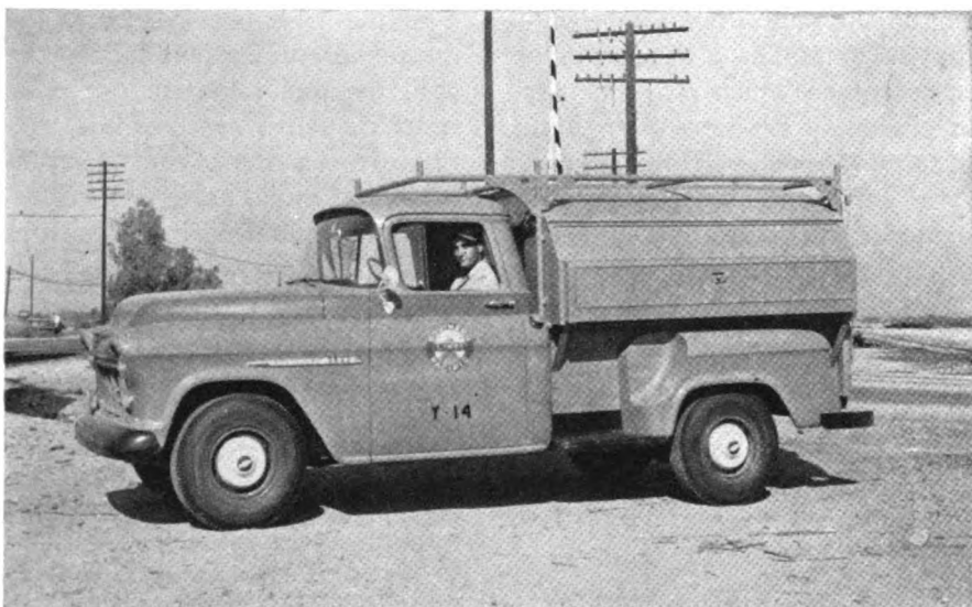
Highway trucks for maintainers cost $30,000 less than installation of motor-car indicators—Territories range from 22 to 28 miles
