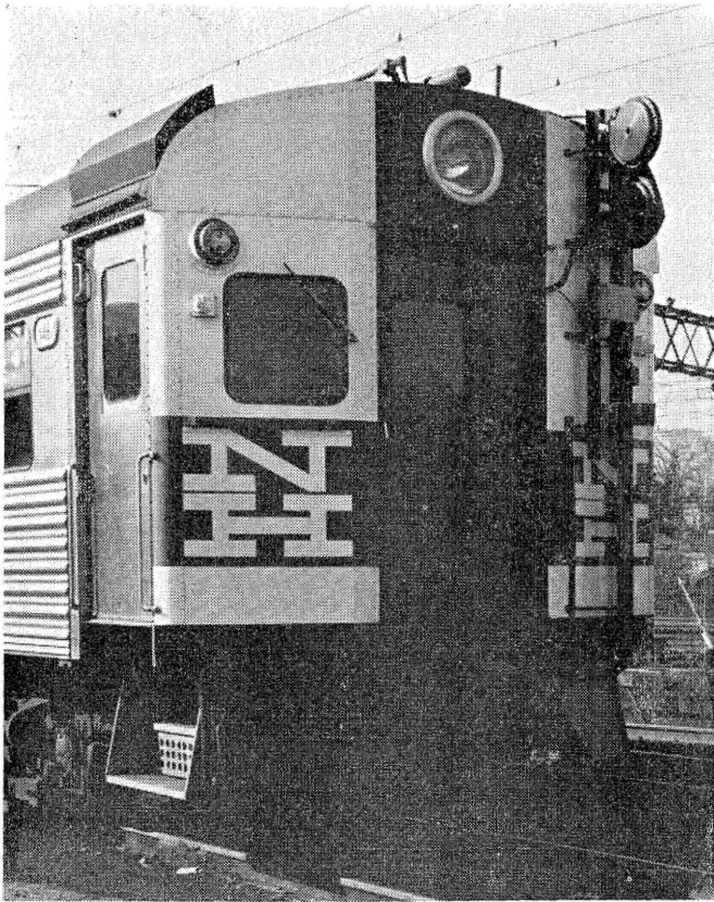
TWO RECEIVING COILS are mounted outside and on the front end of car, shown upper right in this picture
