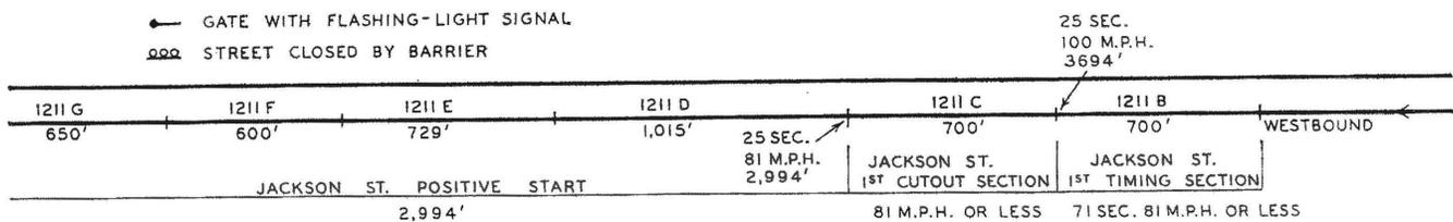
proach sections were occupied but no movement over the crossing was imminent, as for example during switching moves. A watchman, on duty 8 am to 4 pm at Cherry Street crossing, had supervisory manual control of the signals at Clinton, Madison and Cherry. A watchman on duty 8 am to 4 pm at Base Street had control of the signals at Orange, Genesee and Base Streets.
