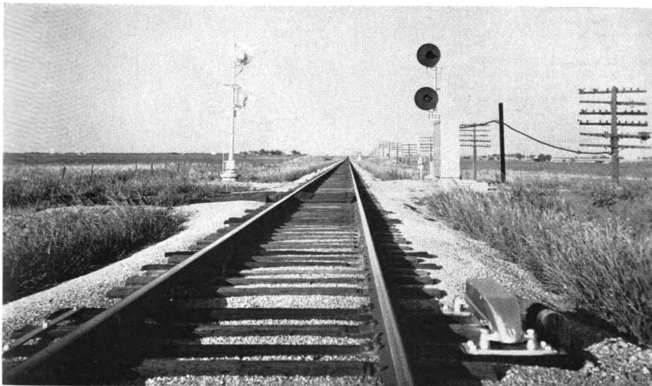
TRAIN STOP INDUCTOR is about 80 ft in approach to each main-track signal
