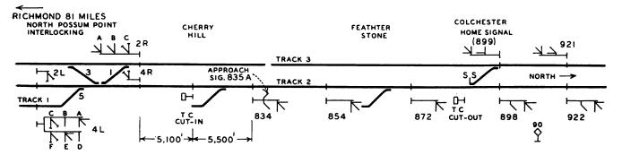
IN ORDER to allow large mechanized track crews to work continuously for eight hours on one track of a section of double track without being required to clear the track for trains, the Richmond, Fredericksburg & Potomac is using signals to direct trains of both directions to use one track between two existing crossovers which may be 5 to 8 miles apart.
