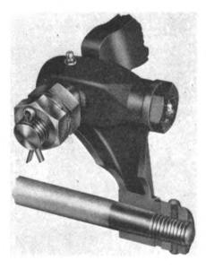
with lock washer, is tightened, the ground tapered surfaces are drawn to a tight fit and are held there so that there can be no looseness to permit wear. A further advantage of the taper fit is that there is no critical place at this end of the rod where vibration could be concentrated to cause a break. These statements have been verified by accelerated tests extending for five months in the New York Testing Laboratories.
