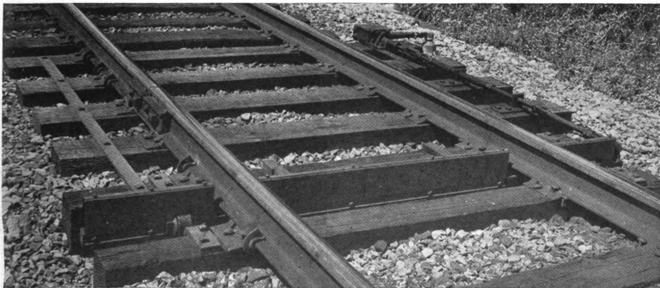
This dragging equipment detector, on the Boston & Maine, is a new type which is directional and self-restoring
