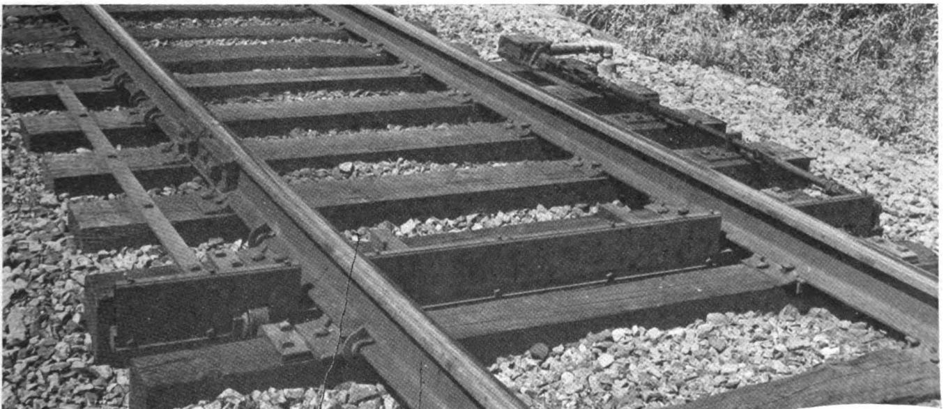
This dragging equipment detector is a new type which is directional and self-restoring
