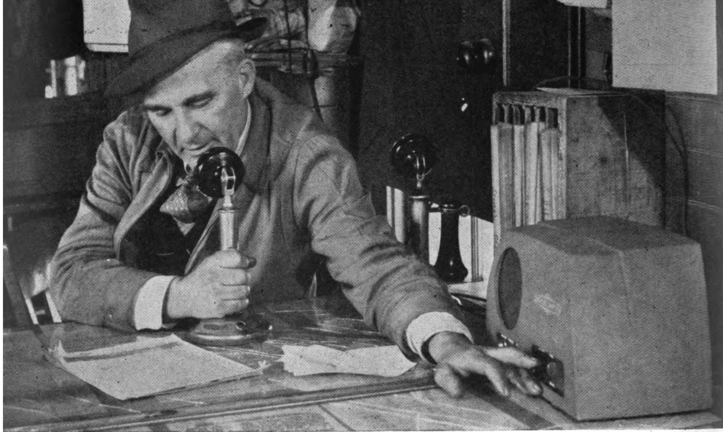
Western Avenue yardmaster giving instructions by radio to crew of radio-equipped switcher. Radio control unit is at right
