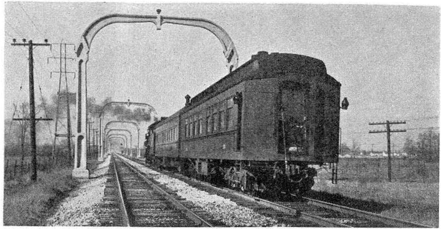
Radio-equipped steam locomotive No. 106 on northbound train in section of double-track territory between Flat Rock and Dearborn where there are concrete arches
