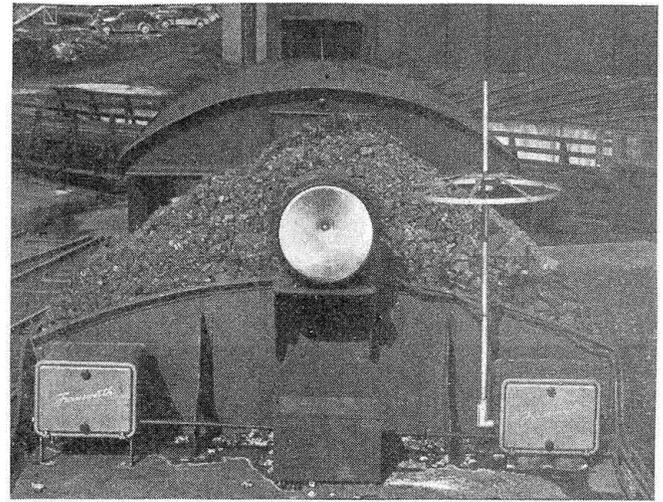
Right — Mounting of radio equipment and antenna on tender of locomotive No. 106
