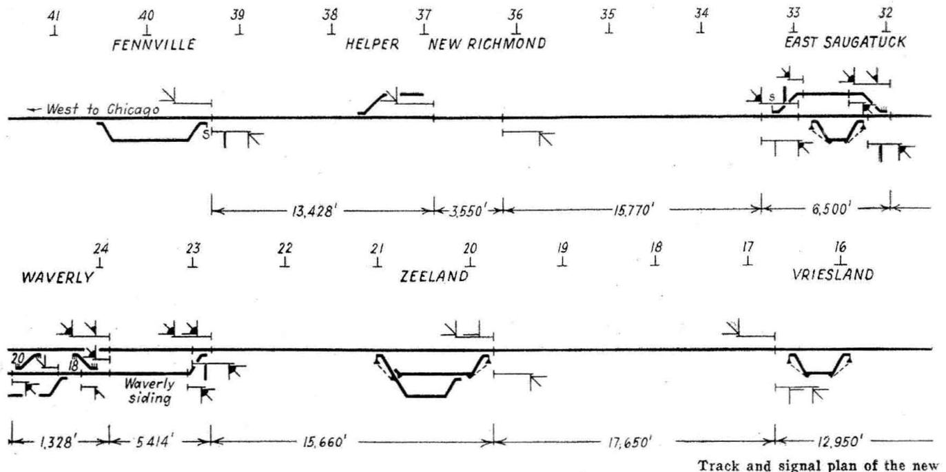
freight trains which are to set out or pick up are run in on the long siding to do this work, thus leaving the main track clear.
