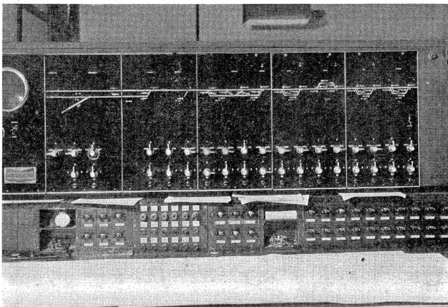
This C.T.C. machine is one of the two which control a 117-mile territory on the D. & R. G. W.
