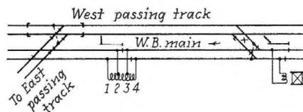
could not be shunted except by bridging the joint that separates their connection to the track, and it was this energy which, when transmitted to the passing track, caused the trouble in the manner explained. It will also be seen that by making leads 2 and 3 common to both directions of feed, the energy feeding west
