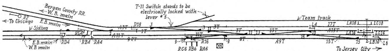
Track and signal plan of new interlocking at Rutherford Junction
