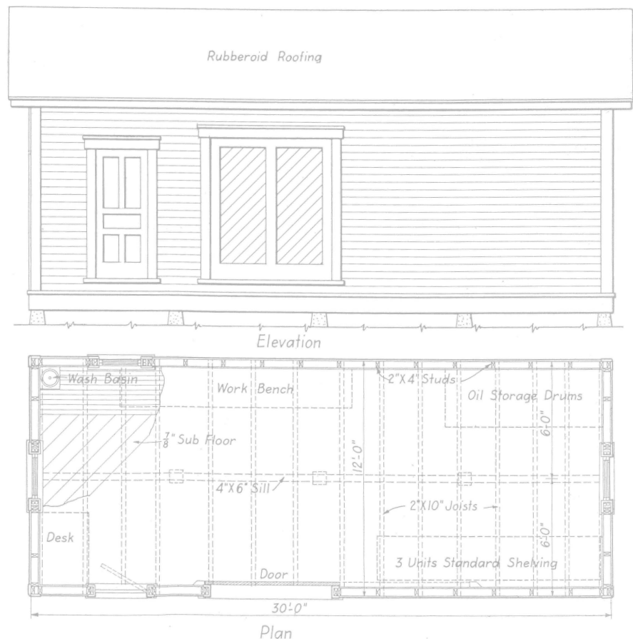
This type of tool house, in use on the Atlantic Coast Line, provides ample space for all storage, motor-car, and office requirements of the maintainer
