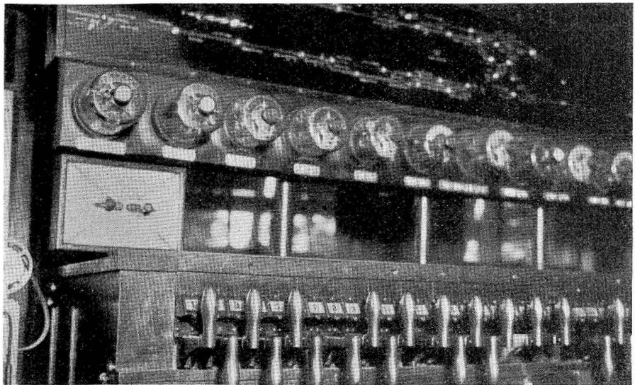
A special interlocked controller for the turn-table signals is mounted at the left of the machine
