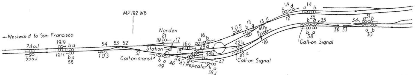
Track and signal plan of Norden interlocking
