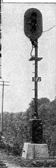
Color-light signal as facing point protection for spring switch. Signal is 150ft. in approach at switch point
