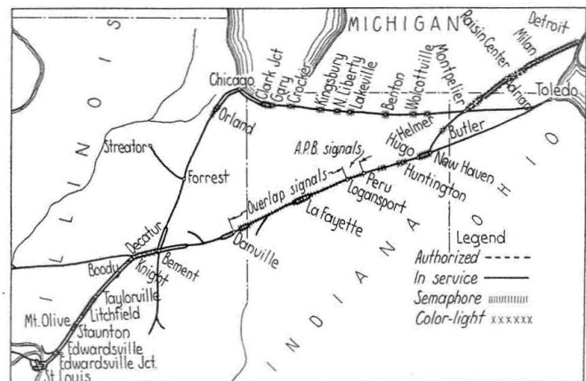
Wabash main line between St. Louis, Chicago and Detroit showing principal automatic block and station signaling
