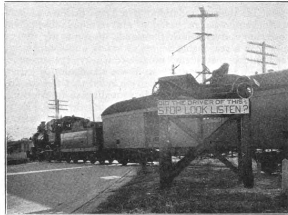
The New Crossing Sign Used by the San Antonio & Aransas Pass to Reduce Grade Crossing Accidents
