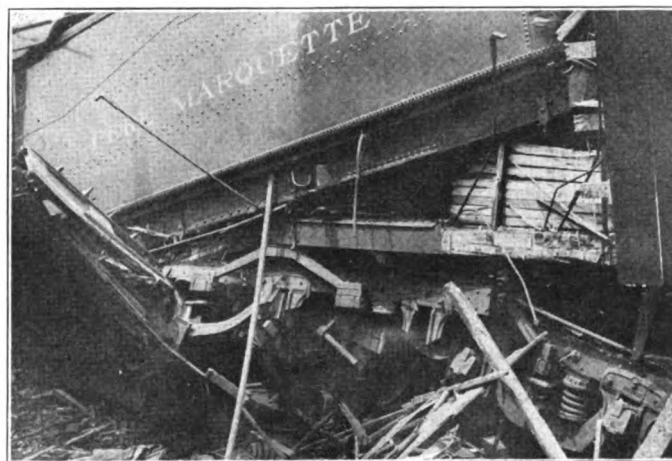
Front End of Baggage Car Telescoped on Tender
