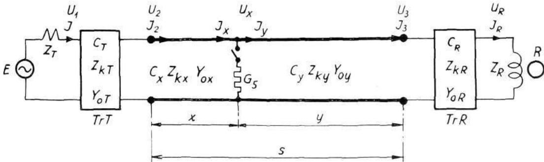
The shunt line equation for a point located  $x$  km from the feed end and  $y$  km from the relay end is obtained as above in section III. The track phase current  $I_{RC}$  for the assumed basic value of the leakage and unoccupied track is divided by the track phase current  $I'_{RD}$  for an arbitrary leakage and shunted track.
