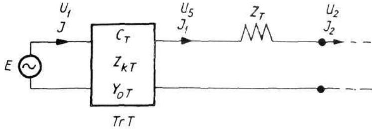
shunt line equation for an arbitrary point of the track we consider the track circuit divided into two parts as in Fig. 17.  $C_x, Z_{kx}, Y_{ox}$  and  $C_y, Z_{ky}, Y_{oy}$  designate the line constants for the sections  $x$  and  $y$  respectively.  $U_x$  is the track voltage at the shunting point.  $I_x$  and  $I_y$  are the current values immediately before and after the shunting point.
