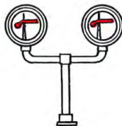
FIG. 2 BLOCK OCCUPIED IN BOTH DIRECTIONS
