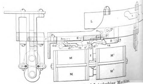
Fig. 11.—“Lever” of Interlocking Machine.
