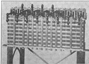
Fig. 10.—Front of Taylor Interlocking Machine.
