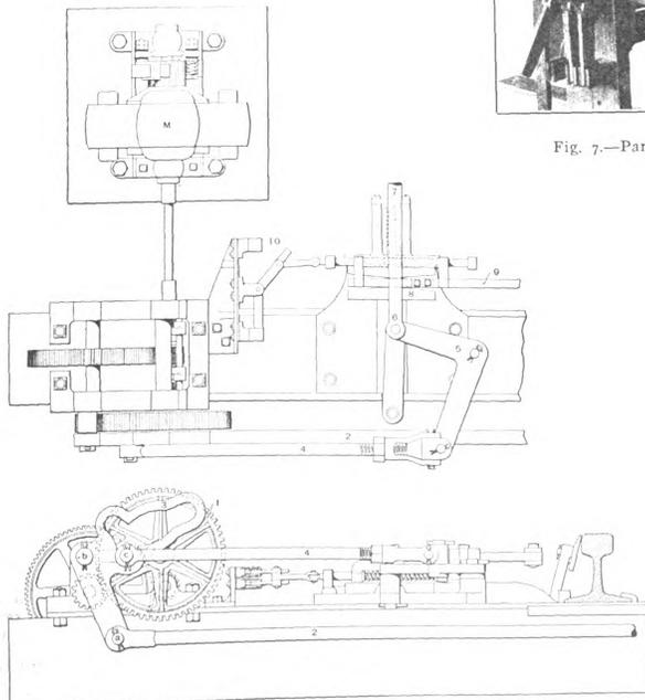
Fig. 2.—Plan and Elevation of Electric Motor for Switch.
