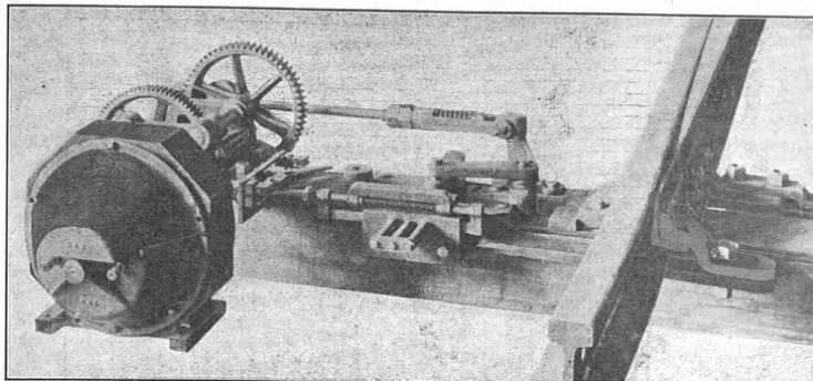
Fig. 3.—Switch Machine (Left Hand).
